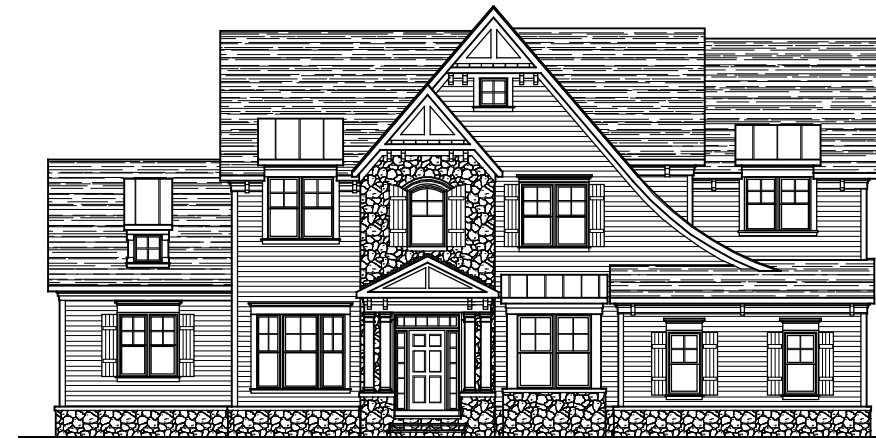
FRONT ELEVATION ELEVATION #7A W/ SIDING AND STONE FRONT 01-17-18 STONE IS OPTIONAL
