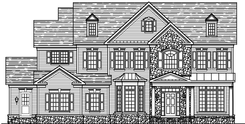
FRONT ELEVATION ELEVATION #12B SIDING AND STONE
