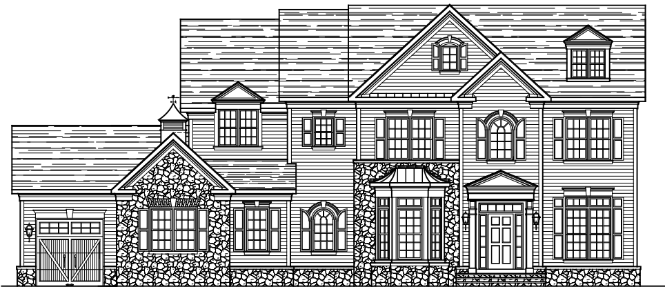
FRONT ELEVATION ELEVATION #4 W/ STONE AND SIDING 08-29-2019
