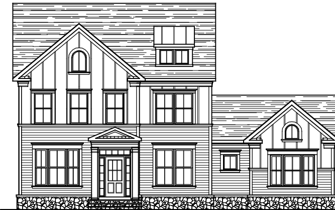
FRONT ELEVATION ELEVATION #7A STONE IS OPTIONAL 05-18-20 W/ BOARD AND BATTEN SIDING (OPTIONAL BLACK WINDOW SASHES & FRAMES)
