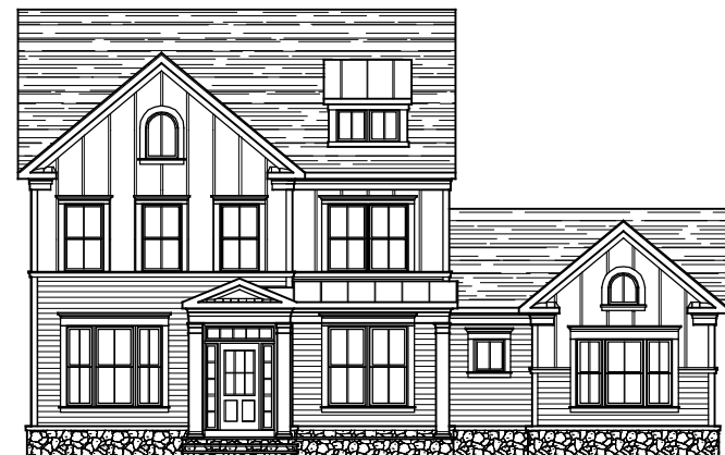
FRONT ELEVATION ELEVATION #7B STONE IS OPTIONAL 05-18-20 W/ BOARD AND BATTEN SIDING (OPTIONAL BLACK WINDOW SASHES & FRAMES)
