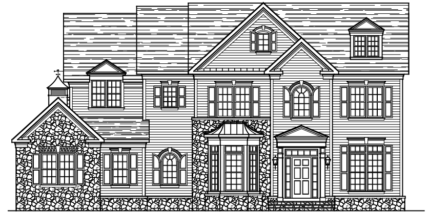
FRONT ELEVATION ELEVATION #4 W/ STONE AND SIDING
