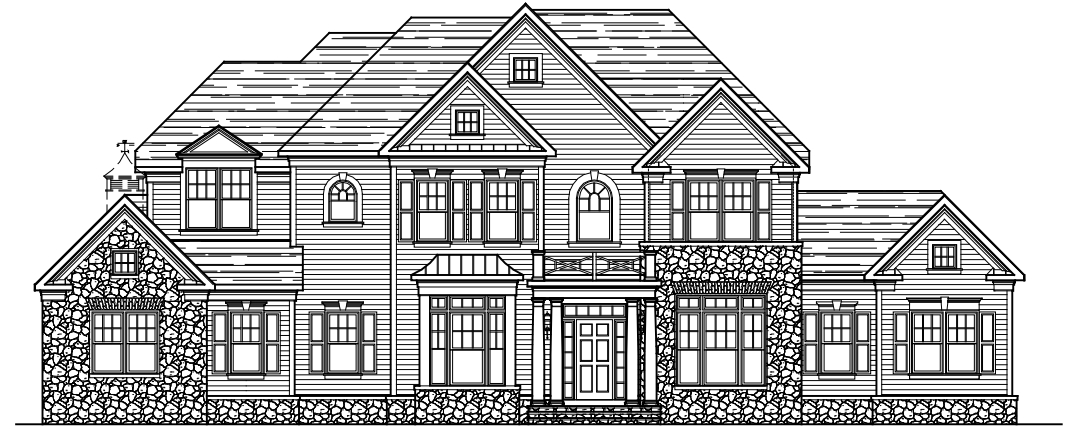
FRONT ELEVATION ELEVATION #5A SIDING AND STONE 08-30-21
