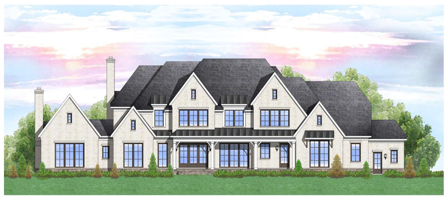
Elevation 4B - brick with stone water table
