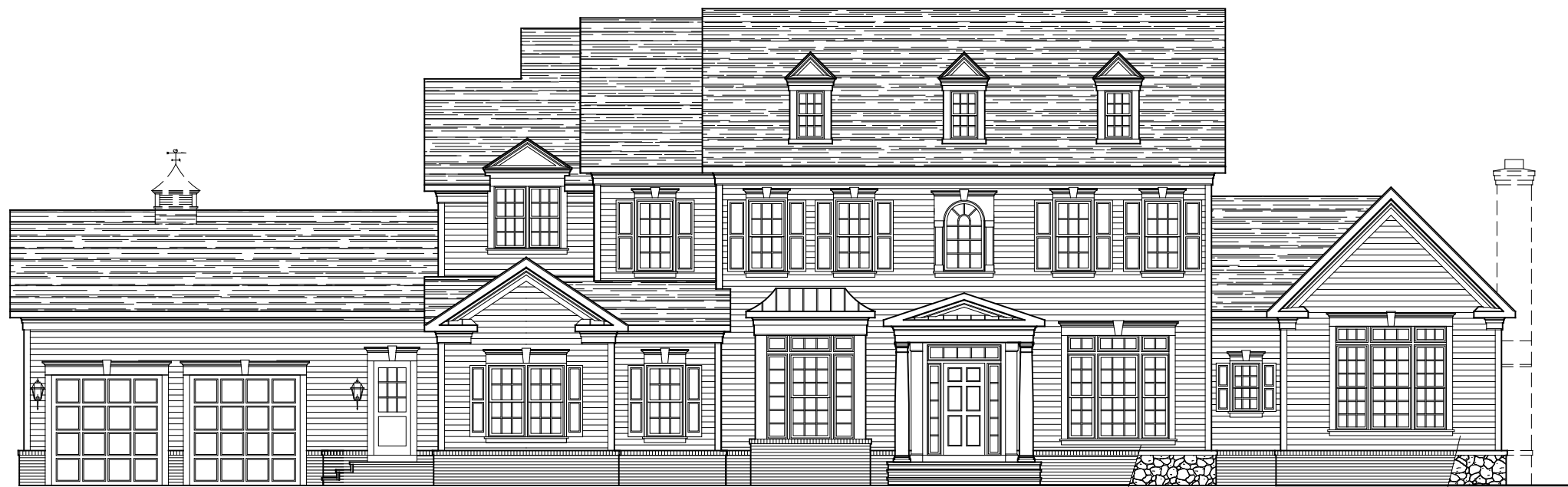
FRONT ELEVATION * ELEVATION #14A W/ FRONT LOAD 2-CAR GARAGE W/ CLUB ROOM STONE IS OPTIONAL 08-22-22
