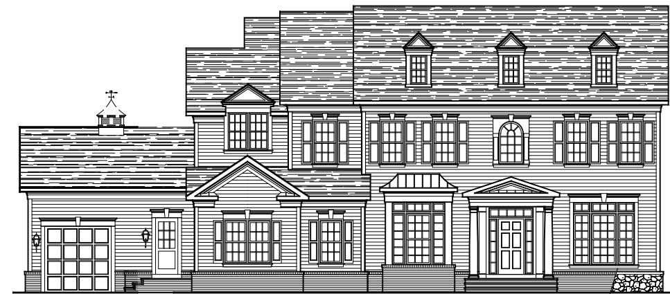
FRONT ELEVATION * ELEVATION #14A W/ FRONT LOAD 1-CAR GARAGE STONE IS OPTIONAL 08-22-22
