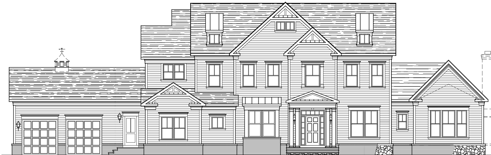
FRONT ELEVATION * ELEVATION #5A W/ FRONT LOAD 2-CAR GARAGE W/ CLUB ROOM STONE IS OPTIONAL 08-22-22
