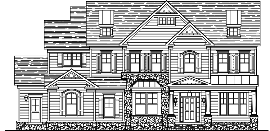
FRONT ELEVATION * ELEVATION #4B W/ SIDING & STONE 08-22-22
