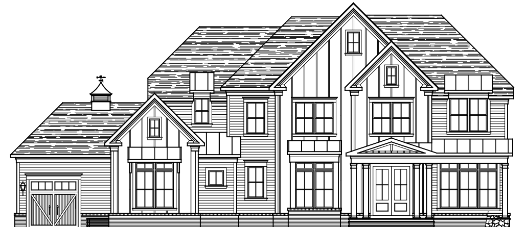
FRONT ELEVATION ELEVATION #6B 09-08-2023 W/ BOARD & BATTEN
