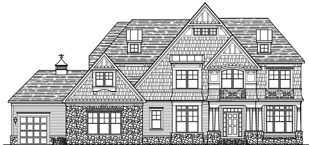
FRONT ELEVATION ELEVATION #9B 09-08-2023 W/ SIDING & STONE
